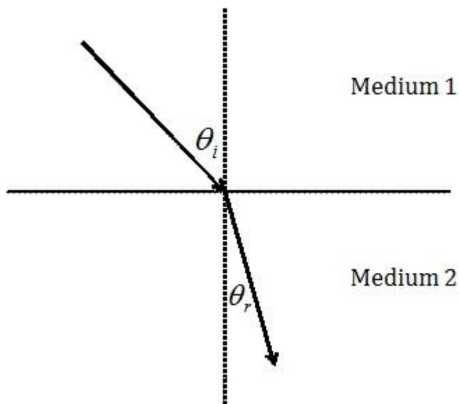
$\theta_i$  and  $\theta_r$  are incident and refracted angles respectively. Which of the following is true for the refractive indices for medium 1 and medium 2? (Perpendicular dotted line represents normal to the interface)
