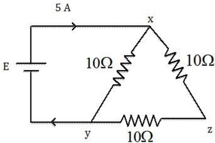
What is the value of E (source voltage), if the current flowing through the circuit as shown above is 5 A?
