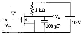
Draw the equivalent circuit and calculate the time taken for the output to fall to 5 V.
