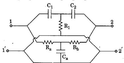
(c) For the network shown below, obtain the Z-parameters. Is the network reciprocal?
